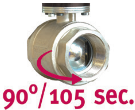
Slow ball valve rotation to avoid "water-hammer" when opening and closing of the valve
