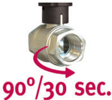
Slow ball valve rotation to avoid "water-hammer" when opening and closing of the valve
