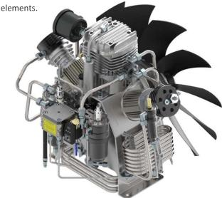
The bearings of the crankshaft have rollers, extremely robust and made in Europe which guarantee a long life of the compressor. An oil pump provides a constant lubrication of the inner workings of the block with oil cleaned of impurities by a filter and by a magnet which catches any metals present in the lubricating oil.
