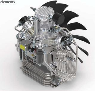
The bearings of the crankshaft have rollers, extremely robust and made in Europe which guarantee a long life of the compressor. An oil pump provides a constant lubrication of the inner workings of the block with oil cleaned of impurities by a filter and by a magnet which catches any metals present in the lubricating oil.
